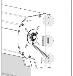
**02** • Based on the existing holes in the support plates, mark the locations for drilling.
