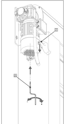
To open or close the door manually, simply push and hold the release lever (10), and use the hexagonal handle 6mm (17) to turn the screw installed in the bottom of the motor, as shown on the image.
