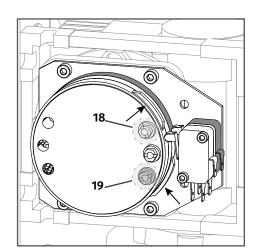
**NOTE** • The red ring must activate the microswitch underneath, and white ring must activate the micro-switch on top, as visible in the left image.
