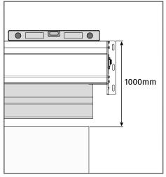
**01** • Apply the safe profile on the wall, centered with the passage. Adjust the safe profile position taking into account the size indicated on the image and the horizontal leveling (use a level).
