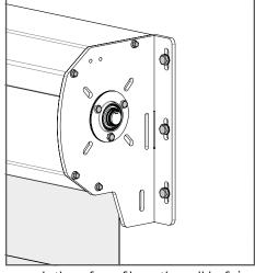
**03** • Make holes in the marked locations, and then apply the safe profile on the wall by fixing it with bushings (metallic) and screws.
