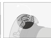
Disassemble the motor from the compact mounting accessory. Just open the tabs as shown in the figure in order to release the motor.
