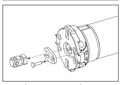
Loosen the screw to remove the support square shaft.
