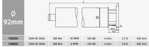
Standard Model- Motor with mechanical limit switch, without handle and without control board. FRA Model- Motor with built-in control board. MT Model- Motor with handle to manually open / close.
