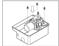
2 • Insert the ball in the pin located on the box and fit the gate anchorage lever (L1).
