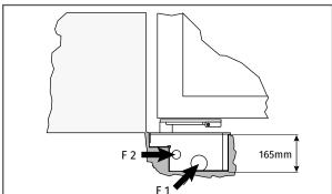
Note: while positioning the box, keep in mind the minimum distance there must be between the pillar and the centre of rotation of the gate hinge.
